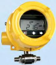
As Safety Instrumented Systems (SIS) grew beyond the process plant into field applications, operators often lacked the infrastructure to support a safety system. UE developed the SIL-certified One Series Safety transmitter to allow direct control of a final element without the need for a SIL certified SCADA, PLC, or RTU, while also supplying the data needed from a 4-20 mA transmitter.
