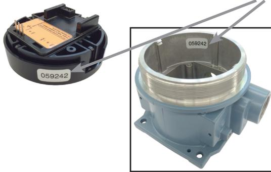
**NOTE:** Do not replace the One Series display module or pressure sensor. Swapping these amongst devices will cause a mis-match between the stored sensor calibration data and the pressure sensor. For proper operation, the display module serial number must always match the serial number inside the enclosure (See Figure 12).
